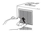
Remove the old filter and install the new filter.
